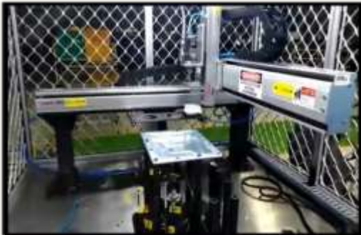
Robot Dispensing Cells Cartesian/SCARA Robot based cells for Glue Dispensing
