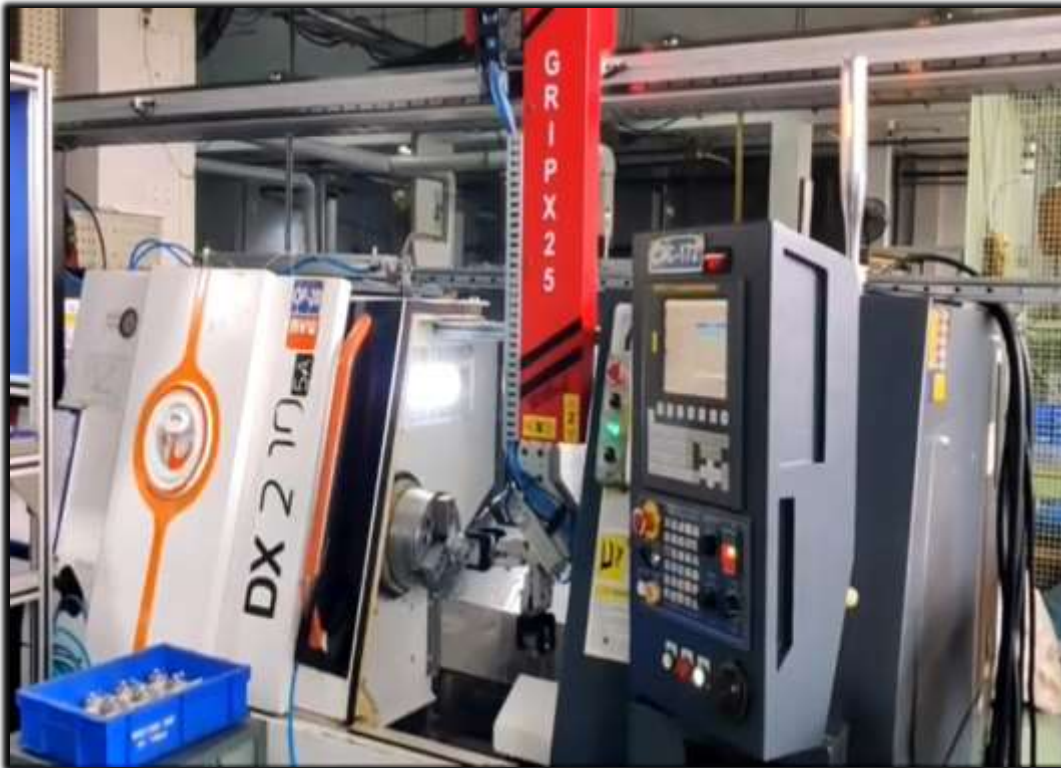
Machine Tending Robot with CNC turning Centre GRIPX 25
