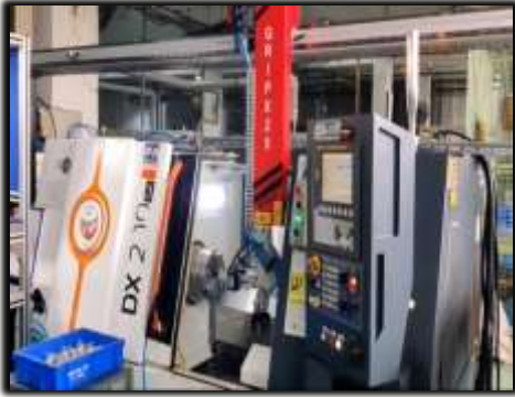
Machine Tending Robots (MTRs) GRIPX 25 for CNC turning centres
