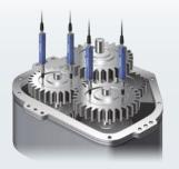
**Transmission parts** height measurement
